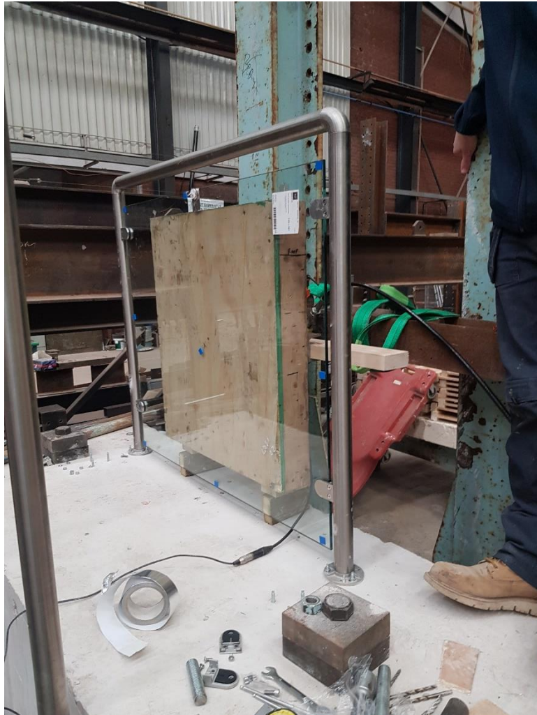
Plate 2 - General Test Configuration Uniformly Distributed Load
